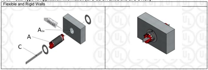
A.4.5 Seal Type 1b Application Information (CFS-SL GA M/L & CP 619 T/CP 617 and CFS-P BA)
