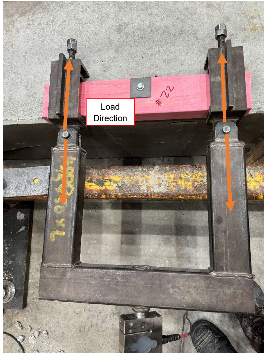
Figure 5 Out of plane shear testing set up
