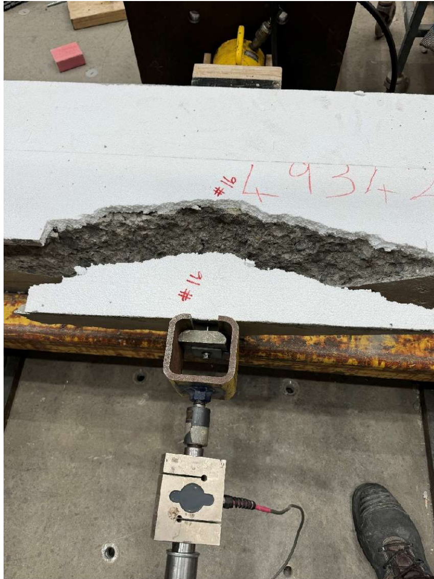
Figure 8. Failure by concrete edge breakout during tension testing.
